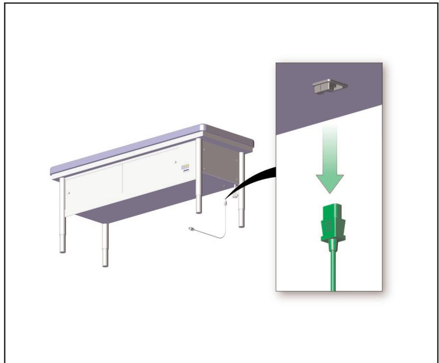
**Step 4--** Remove fuse holder from appliance inlet, as shown in Figure 4.8.4.
