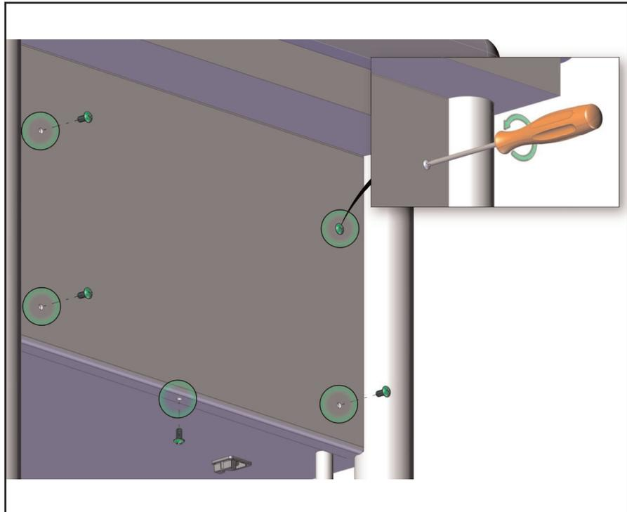
**Step 5--** Remove the cover from the motor enclosure, as shown in Figure 4.7.5. Any repair should be performed by trained or certified service personnel.
