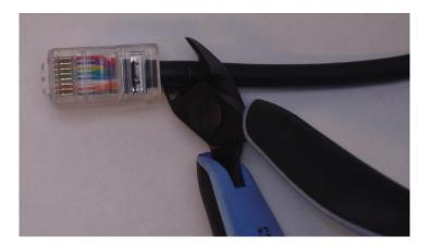
Cut off the cable near the control panel. Use the used cable to thread the new control panel cable through the steel profile.
