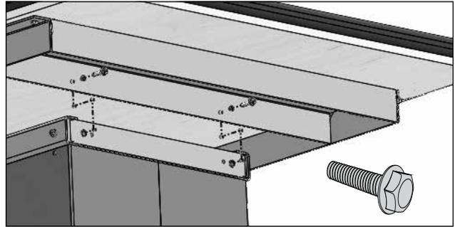
**6** Working on just one end, elevate the top using help and align the holes on the top with the holes in the base. Insert the bolts removed from the shipping supports and finger tighten. DO NOT FULLY TIGHTEN.
