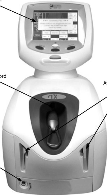
The Base Unit serves to house the mechanical and electrical components that provide the actual traction tension for the TX traction unit under the electronic control and supervision of the Controller.
