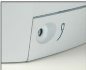
1. Attach the Patient Interrupt Switch by inserting the male end of the cable into the Patient Interrupt Switch Receptacle located on the front of the unit.
