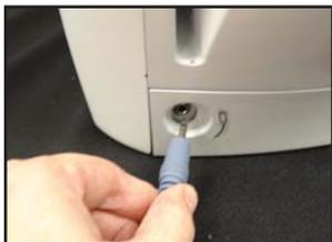
Turn the unit off. Disconnect the traction unit from its power source. Disconnect the Patient Interrupt Switch from its receptacle.
