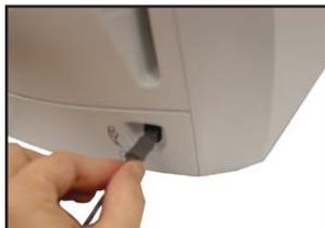
Plug the sEMG lead wire into the front of the unit.
