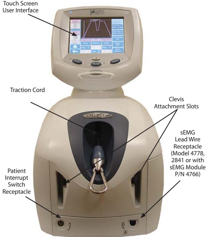
The Base Unit serves to house the mechanical and electrical components that provide the actual traction tension for the Triton traction unit under the electronic control and supervision of the Controller.
