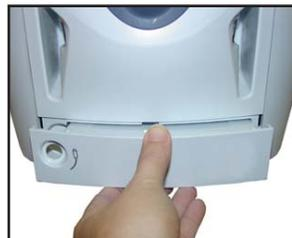
Gently push the front panel back into the front of the traction unit. Once the plastic of the unit and the front panel are aligned, the connector should be inserted properly, with the tabs locked in place.
