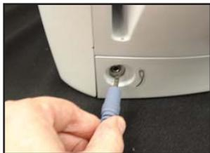
Turn the unit off. Disconnect the traction unit from its power source. Disconnect the Patient Interrupt Switch and the sEMG lead wire from the receptacles.
