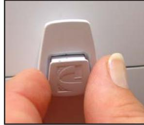
Insert the Patient Interrupt Switch Hook Cover to cover the hook screw hole.
