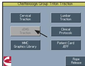
The traction unit should automatically recognize that the sEMG Module has been removed, with the sEMG Traction button now being inactive on the Home Screen.
