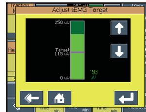
**To Adjust the Manual Target** - Press the Target button until Manual is selected, press the Adjust Target button, press the Up or Down Arrow buttons to adjust the Target to the prescribed level, and press the Return Arrow to accept. The target range is from 5 to 2,000  $\mu$ V.
