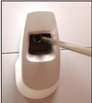
Place the Patient Interrupt Switch Hook over the screw hole and tighten the Hook Screw in place.
