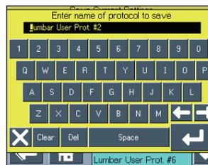
After the Return Arrow is pressed, a keyboard will be displayed to enter the name of the User Protocol. Once the User Protocol name has been entered, press the Return Arrow to accept.
