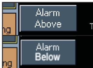
**Alarm button** - This button allows the clinician to choose if the alarm should sound above or below the target.
