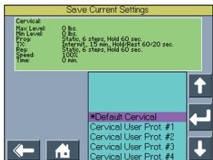
Press the Up or Down Arrow button to select the number of User Protocol to save the desired treatment to or the Default Protocol button to save treatment as the default. Press the Return Arrow to accept.
