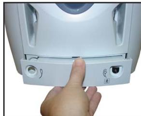
Gently push the sEMG Module into the front of the traction unit. Once the plastic of the unit and the module are aligned, the connector should be inserted properly, with the tabs locked in place.
