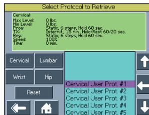
The list of the User Protocols is located on the right side and the body part buttons are located on the left side to toggle between body part User Protocols. Press the Up or Down button to review the User Protocols.
