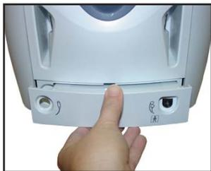
Gently press the tabs underneath the unit, pull and remove the sEMG Module from the traction unit
