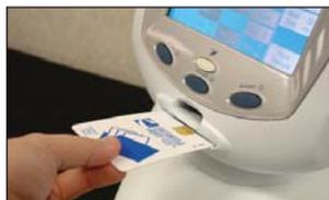
Insert a new Patient Data Card (with the gold chip facing up) into the Patient Data Card port located on the front of the traction unit.
