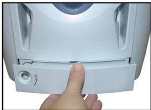
Gently press the tabs underneath the unit, pull and remove the front panel from the traction unit
